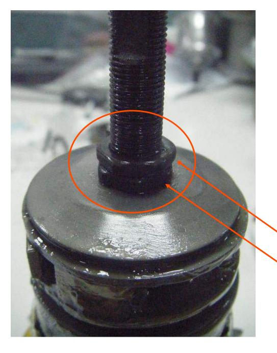
Step 4: Tighten Nut 1 and Nut 2.
