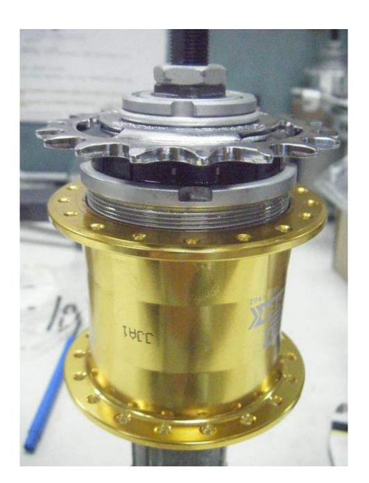
Step 2: Remove Internal. No proprietary tool is needed. Use a hammer and punch, hook spanner, or adjustable spanner to drift internal out. Left
