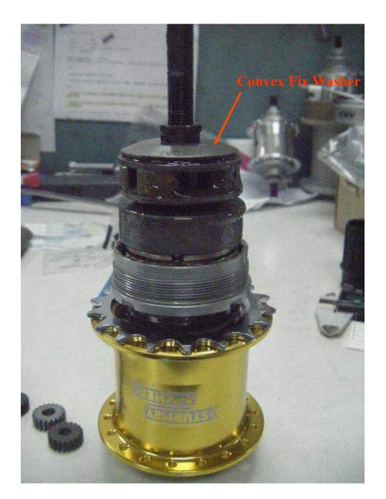
Step 3: Hold Axle securely, check if Convex Fix Washer is loose.
