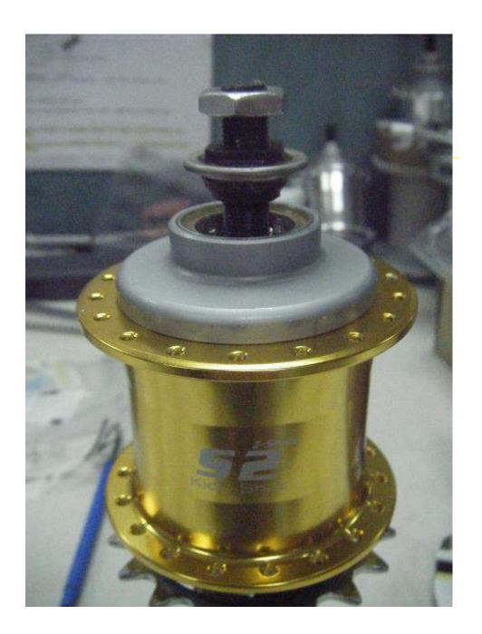
Step 1: Remove LH Nut And Cone
